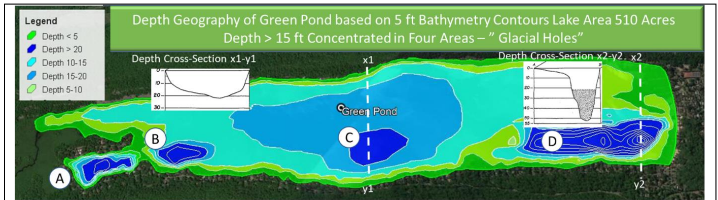
Figure 3.2: Bathymetry and depth cross sections show Green Pond's classical glacial "hole" character
